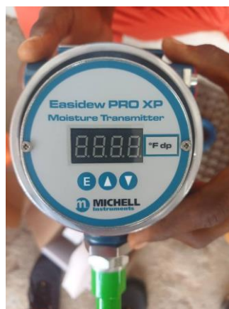
Michell Easidew PRO XP dew-point transmitter
